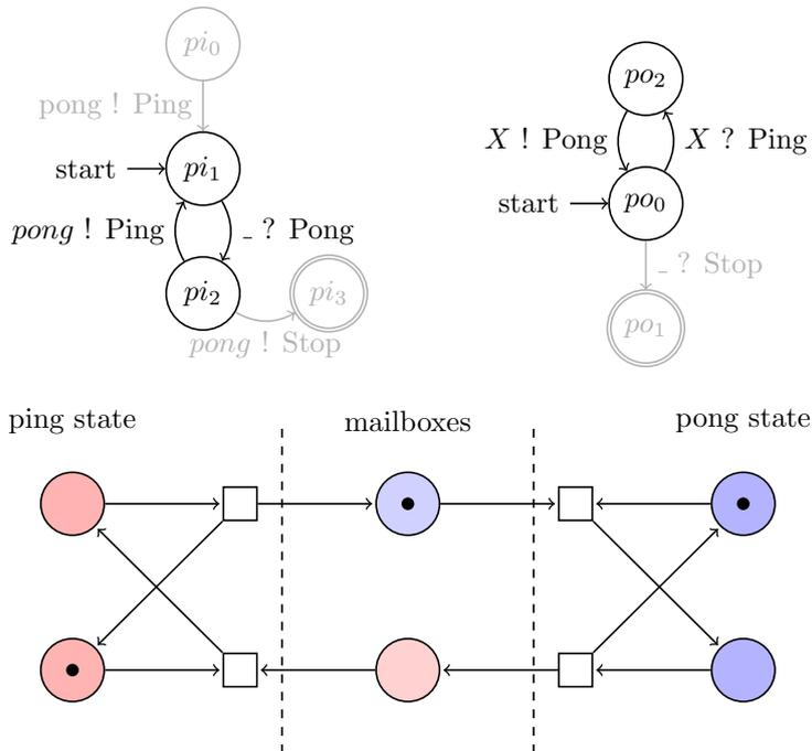
Figure 1.3: Petri net corresponding to a fragment of the ping-pong example
